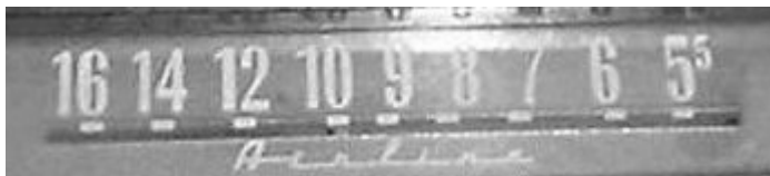
Nonlinear indicator dial for selecting frequency in an old manually-tuned AM radio
